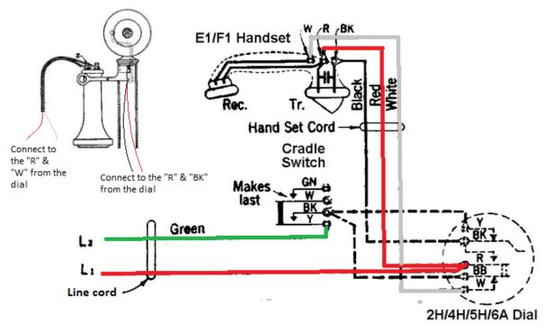
This schematic was created to show how to wire a Western Electric telephone (Candle Stick, 102 & 202) without a subset box. Obviously there is not a bell or Anti-Sidetone Induction Coil. By wiring a telephone without the coil, you may experience a slight reduction in volume on other extension phone being used at the same time.
