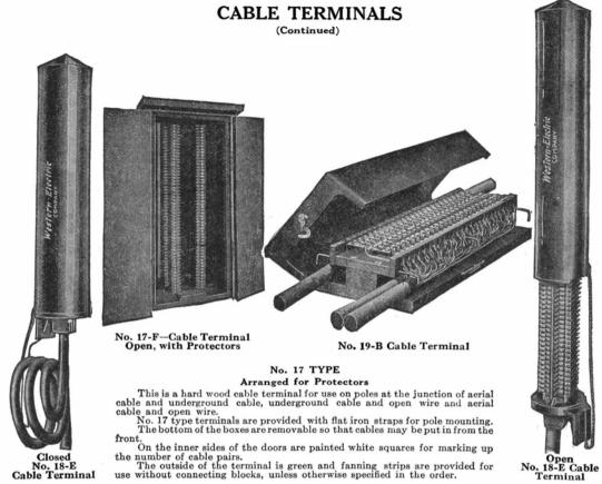
In the No. 17 type terminals the No. 1074A protectors or the No. 17B protectors on the No.1 D, E or F connecting blocks or with the No. 1075A protectors are used.
