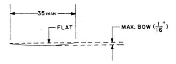
Fig 2—Checking Reel Film for Bow
