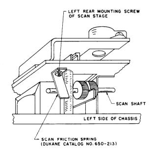
Fig. 1 – Installation of Scan Friction Spring
