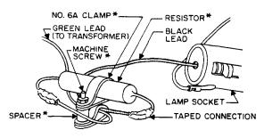
Fig. 2 – Lamp Voltage Modification. Items Marked With an Asterisk (\*) are New Parts. For List ↓ of Parts, see 3.01.
