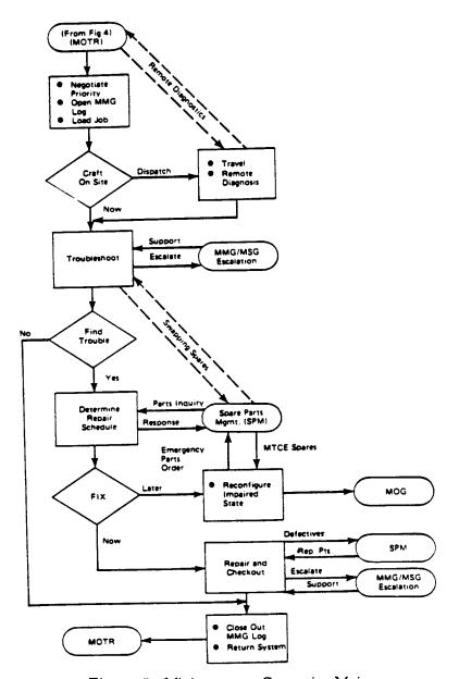
Figure 5. Minicomputer Corrective Maintenance
