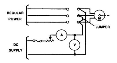
Figure 4. Schematic for Drying a 3-Phase AC Machine While Stationary by Heating with Low-Voltage DC
