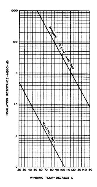
Figure 3. Insulation Resistance of Induction Motors
