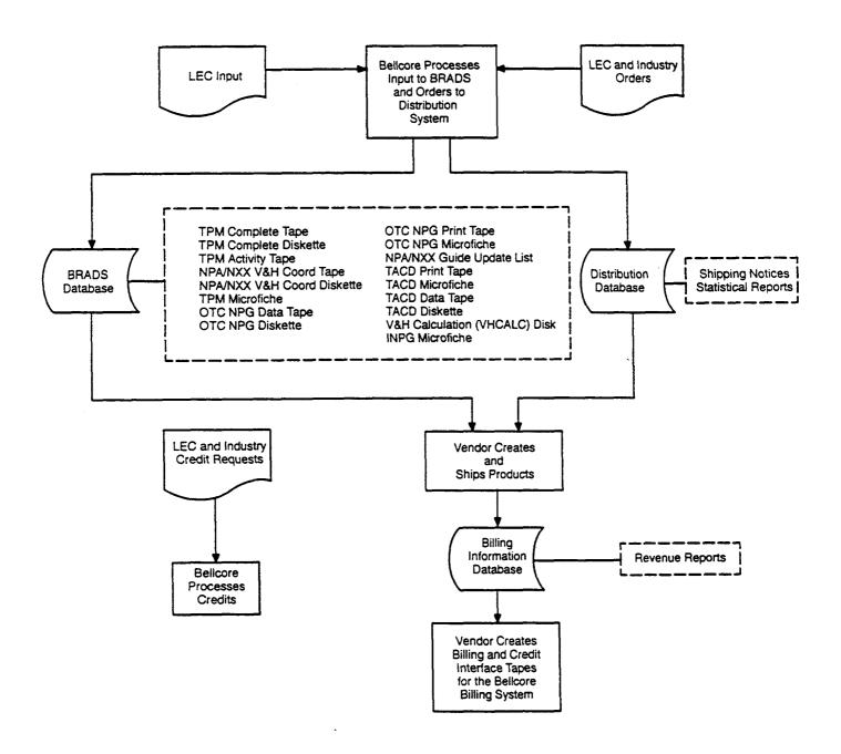
Figure 1-1. BRADS System Diagram
