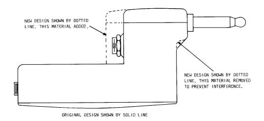
Fig. 2—292-Type Amplifier Showing Difference Between Earlier and Later Models
