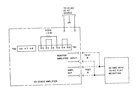
Fig. 2—♦Setup for Noise Test for KS-20425 Amplifier System
