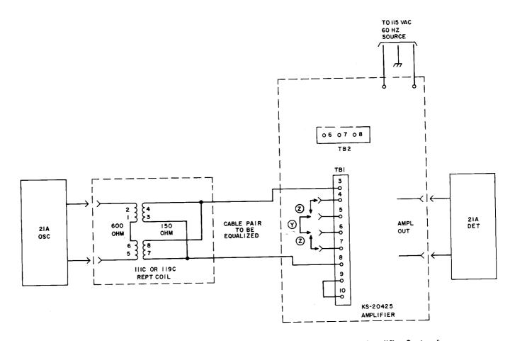
Fig. 3—♦Test Setup for Equalizing a Single Section Using the KS-20425 Amplifier System♠
