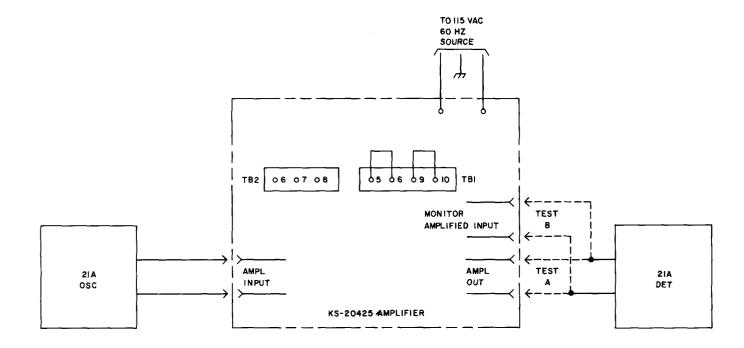
Fig. 1—♦Setup for Gain-Frequency Test for KS-20425 Amplifier System
