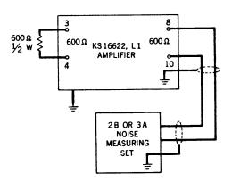
Fig. 3 — Test Setup for Noise Test
