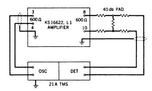
Fig. 1 — Test Setup for Gain-Frequency Test
