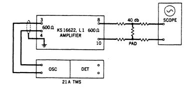
Fig. 4 — Test Setup for Observing Distortion
