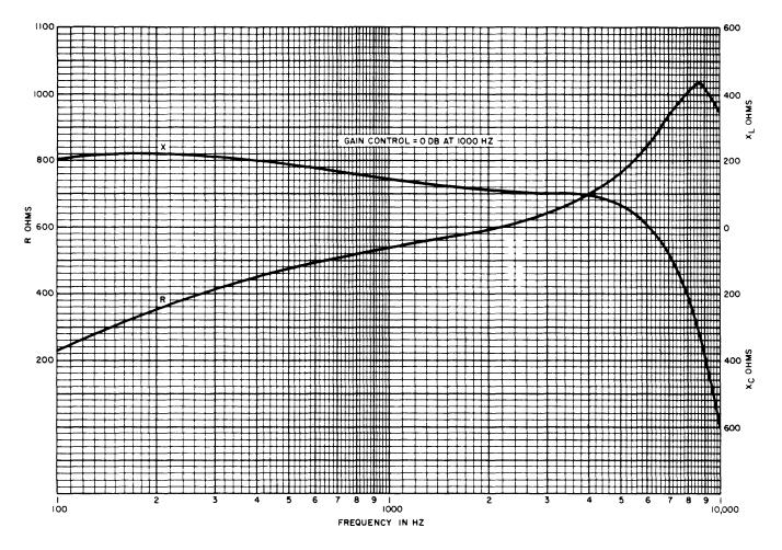
Fig. 4—KS-20378 Amplifier Output Impedance—600-Ohm Termination
