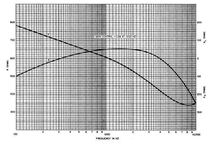
Fig. 3-KS-20378 Amplifier Input Impedance-600-Ohm Termination
