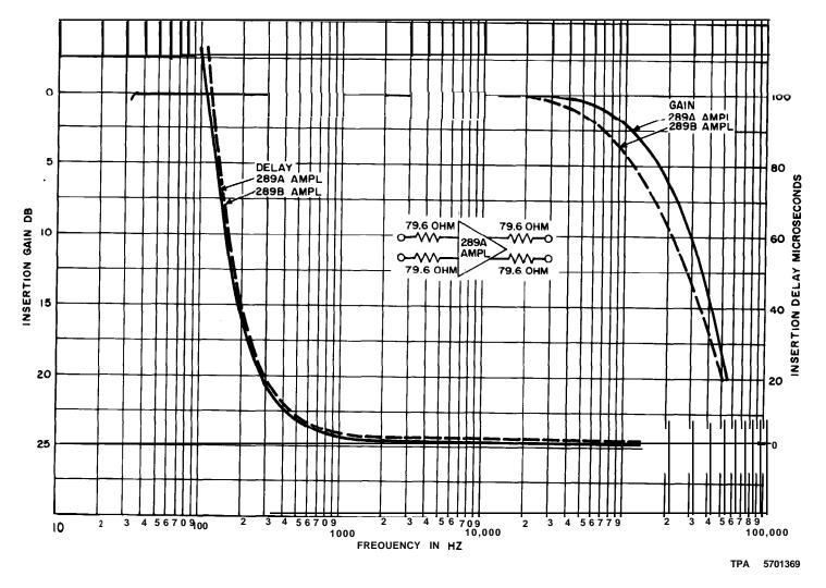
Fig. 6-289A and 2898 Amplifier-Envelope Delay and Gain-Frequency Characteristics
