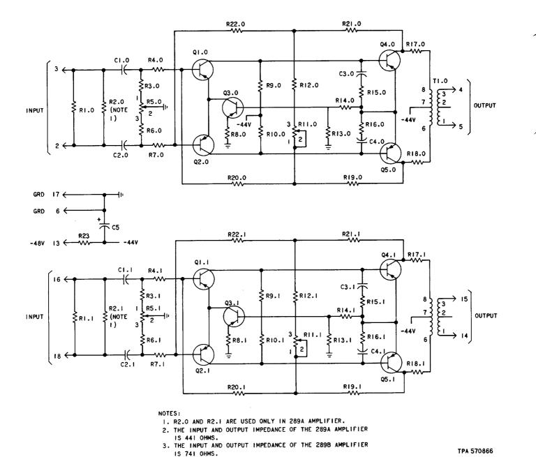
Fig. 3—Schematic Diagram of 289A and 289B Amplifier
