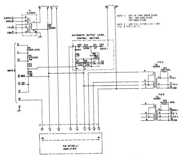
Fig. 6 - KS-16754, List 1 and 3 Amplifiers, Schematic
