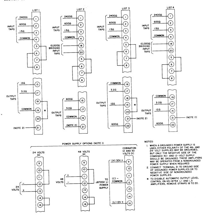
Fig. 4—Connection Data for KS-16754 Amplifier
