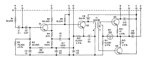
Fig. 3—KS-16728 L1 Amplifier, Schematic
