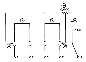
Fig. 5 — Connection Data for Remote Gain Control for KS-16754 Amplifier
