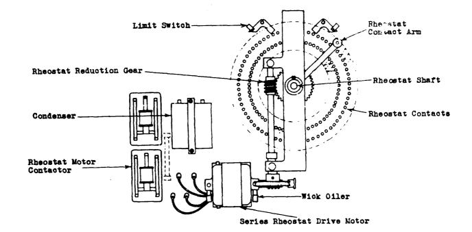
Fig. 6 - Motor-driven Rheostat Assembly
