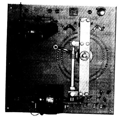
Fig. 2 - D-c Automatic Rotating Cam Type Voltage Regulator KS-5117
