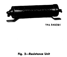
The resistance, when provided, is an enameled tube resistance with a suitable protective guard. It is adjusted at the factory for normal running temperature of the motor whose speed is nominally 2000 rpm. The resistance unit has a number of taps, the proper tap being ascertained and marked at the
