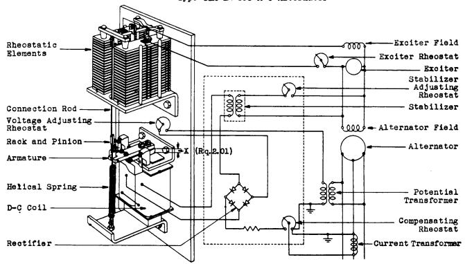
Fig. 3 - Typical Schematic Circuit
