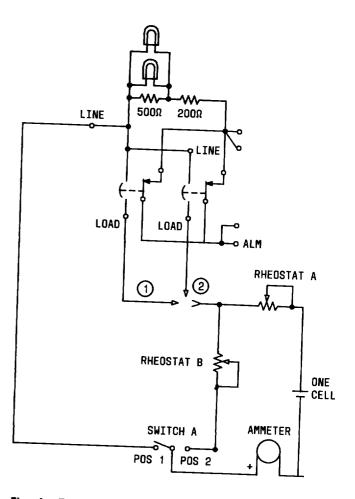
Fig. 4—Test Circuit—Common Line Termination—With Lamp Assembly
