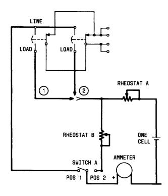
Fig. 6—Test Circuit—Common Line Termination—Without Lamp Assembly
