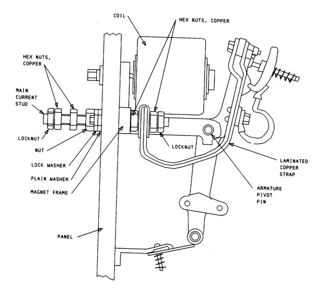
Fig. 5—PTypical Nut and Stud Assembly for Main Current-Carrying Connection€
