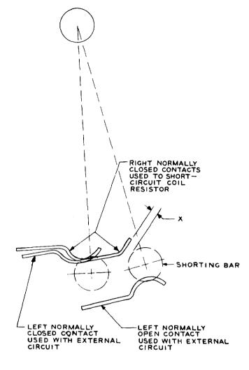
Fig. 4—Auxiliary Contact Arrangement
