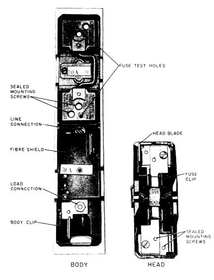
Fig. 1-30-Ampere SAFTOFUSE Unit-Assembly Details
