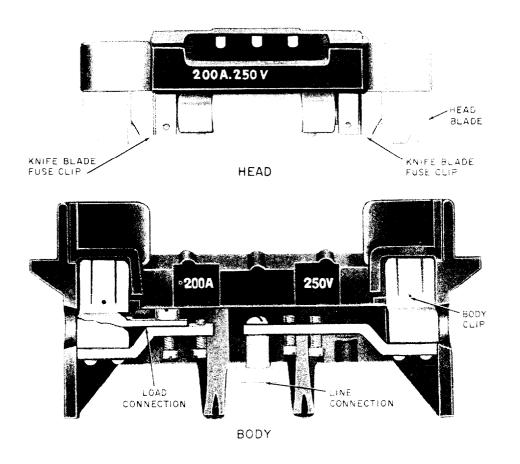
Fig. 2—200-Ampere SAFTOFUSE Unit—Sectional View
