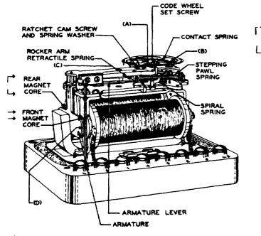
NOTE - THE NOS. SOA AND D-175279 SELECTORS ARE THE SAME AS THE SELECTORS SHOWN ABOVE EXCEPT THEY HAVE TWO RINGING POSITION TERMINALS AND ARE DESIGNED FOR PLUG-IN CONNECTION BY MEANS OF A JACK ON THE UNDERSIDE OF THE BASE.
