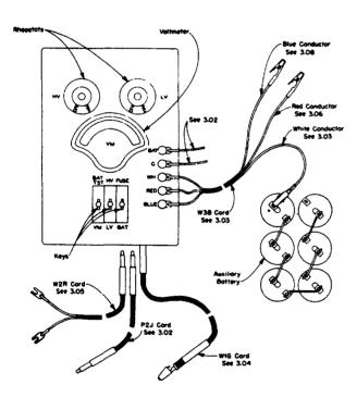
Fig. 1 - Method of Connecting Selector Test Set
