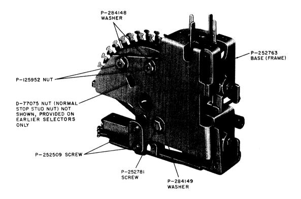
Fig. 1-Bottom View of 204-Type Selector
