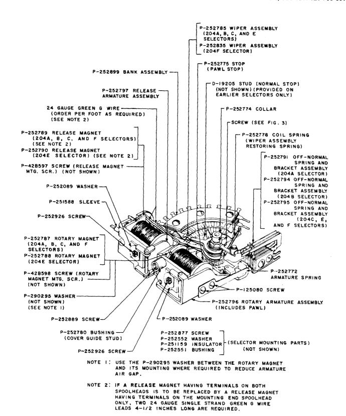
Fig. 2—Top View of 204-Type Selector
