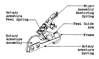
Fig. 4—Location of Rotary Armature Spring and Pawl Guide Arm
