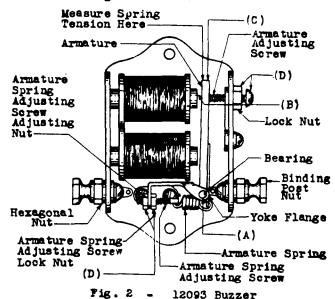
2.06 Operation The buzzer shall give a clear signal when the circuit in which it is used is closed. It is designed to give a clear signal on 20 to 28 volts, inclusive, D.C.
