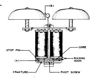
Fig. 3 - Ringers "ithout Armature Stop Screw
