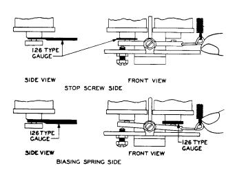
Fig. 6 - Method of Checking Airgaps on Ringers With Stop Screws
