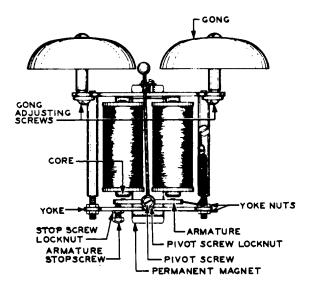
Fig. 11 - Adjusting Screws for 6-, 7-, 8-, and 42-type Ringers
