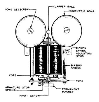
Fig. 13 - Adjusting Screws for 78-type Ringers
