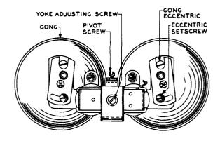
Fig. 12 - Adjusting Screws for Eccentric-type Gong Mountings
