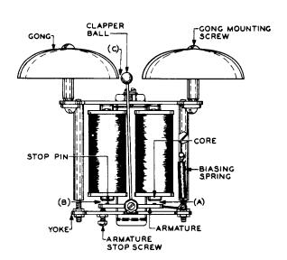
Fig. 2 - Ringers With Armature Stop Screw
