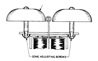
Fig. 14 - Adjusting Screws for B3B Ringers
