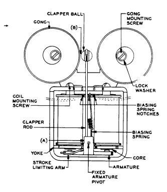
Fig. 4 - Parts of B-type Ringer Except B3B Ringer
