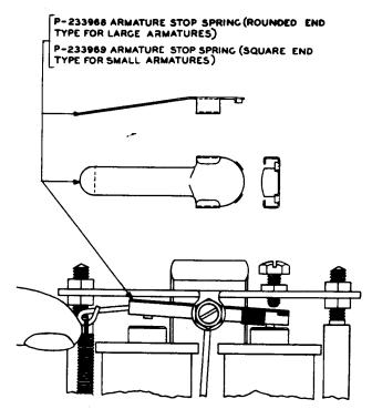
Fig. 10 - Method of Mounting Armature Stop Spring
