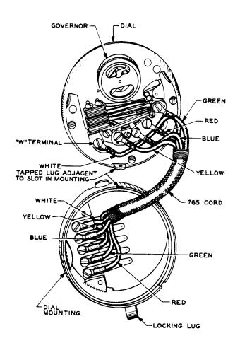
Fig. 6 — Method of Cording Dial Mountings and Dials Having the W Terminal As Part of the Contact Spring Assembly, Using No. 765 and Similar Cords
