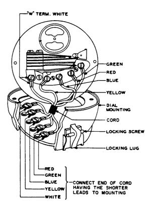
Fig. 1 — Method of Cording Dial Mountings and Dial, Using D5AD or D5AH Cord With Dial Having a W Terminal As a Part of the Contact Spring Assembly (D5AD Cord Illustrated).
