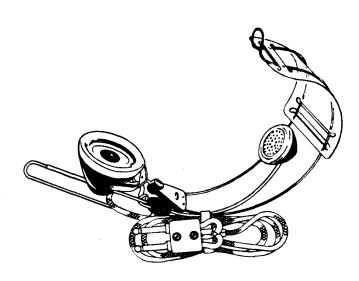
Fig. 2(A) - Cord Equipped With the 289-Type Plug
