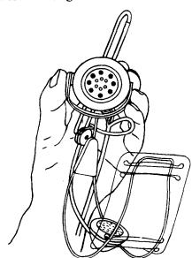
Fig. 1 — Handling the 52-Type Head Telephone Set
