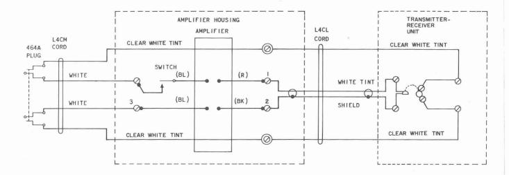
Fig. 8—Amplifier Connecting Diagram
