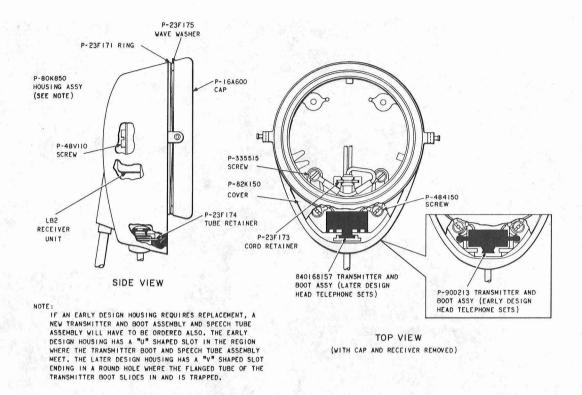
Fig. 3—Receiver-Transmitter Unit
