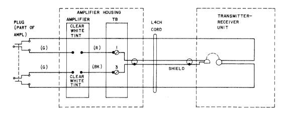
Fig. 9-280A Amplifier Connecting Diagram
