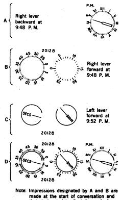
that designated by C at the end of conversation. D shows the completed impression as it appears on the ticket to indicate the elapsed time of 4 minutes and 5 seconds starting at 9:48 P.M.
