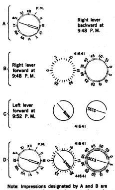
made at the start of conversation and that designated by C at the end of conversation. D shows the completed impression as it appears on the ticket to indicate the elapsed time of 4 minutes and 5 seconds starting at 9:48 P. M.
