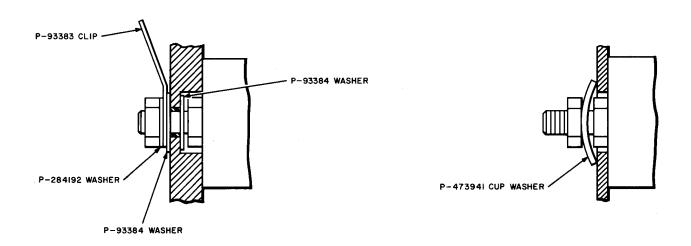
Fig. 8—Mounting Parts for 14-Type Registers Equipped With Spacer
