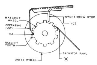
Fig. 1—Typical 14-Type Message Register (Initial Design)
