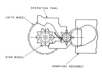
Fig. 3—Typical 14-Type Message Register (MOD 2)
