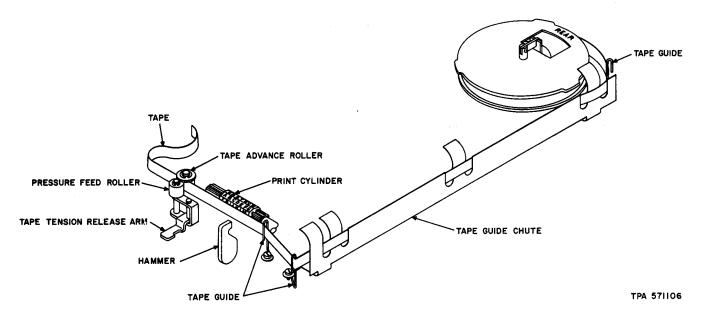
Fig. 3—Method of Threading Tape
