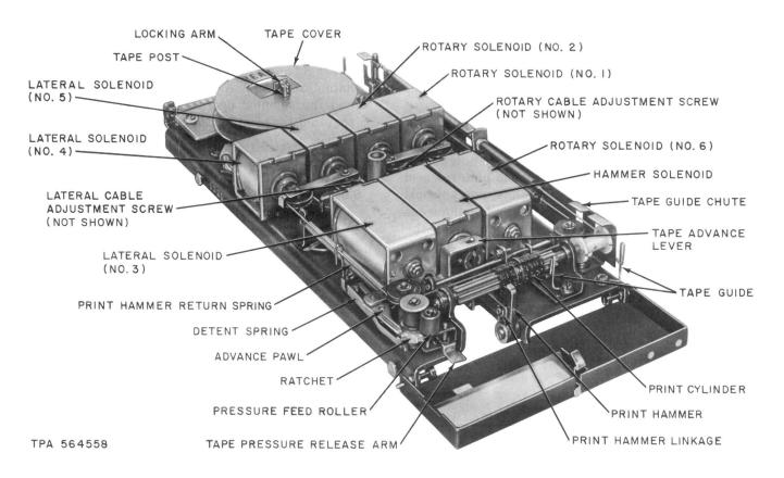
Fig. 2—KS-19717 L6 Tape Printer—Cover Removed
