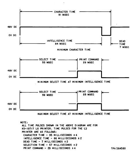
Fig. 8—Pulse Timing Diagram—64 Character Printer
