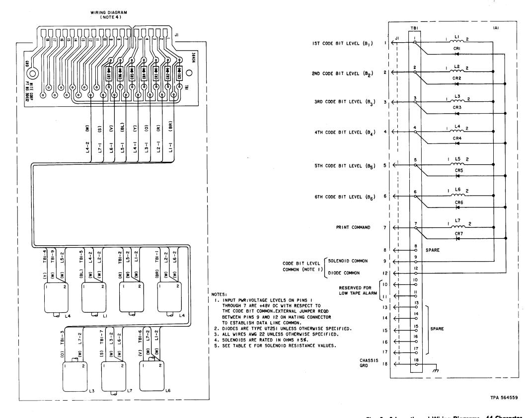
Fig. 5—Schematic and Wiring Diagrams—64 Character
