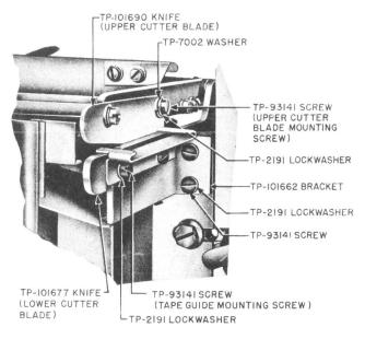
Fig. 7—Cutter Blade and Tape Guide
