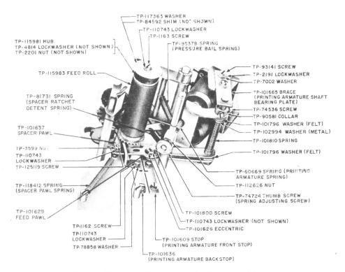
Fig. 6—₱Printing Mechanism (bottom view)♠
