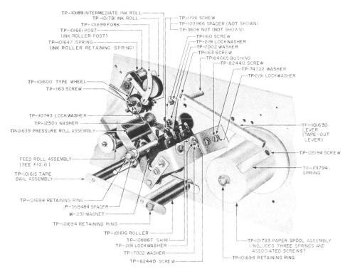
Fig. 5—Printing Mechanism (top view)
