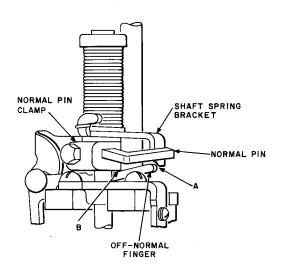
Fig. 5—Normal Pin Clamp and Associated Parts
