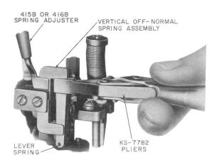
Fig. 17—Method of Adjusting U-Shaped Springs on Vertical Off-Normal Spring Assembly
