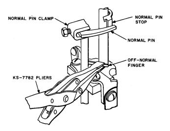
Fig. 23—Method of Adjusting the Off-Normal Finger
