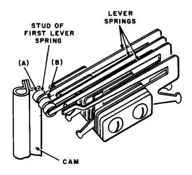
Fig. 9—Relation of Cam Spring Assembly to Cam
