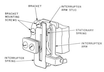
Fig. 19—Bell-Crank-Type Vertical Interrupter Spring
