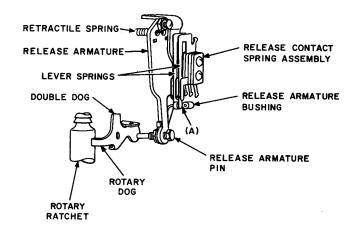
Fig. 11—Release Spring Assembly and Associated
