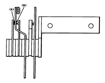
Fig. 2—Rotary Interrupter Spring Assembly with Offset Spring
