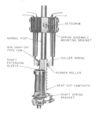
Fig. 28—Normal Post Spring Assembly Having Rubber Rollers Operated by Nonsnap-On-Type Cam (Single Cam Illustrated)
