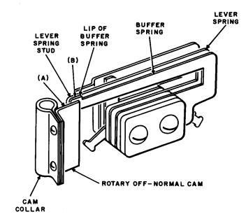
Fig. 10—Illustrating Rotary Off-Normal Spring Requirements
