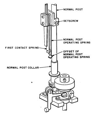
Fig. 31—Normal Post Spring Assembly Operated by Normal Post Collar
