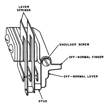
Fig. 7—Vertical Off-Normal Spring Assembly Having
