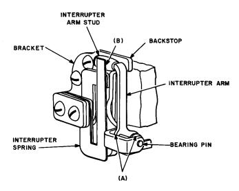
Fig. 3—Bell-Crank-Type Vertical Interrupter Spring Assembly
