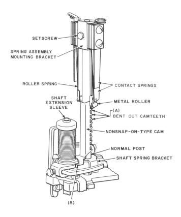
Fig. 13—Normal Post Spring Having Metal Rollers
