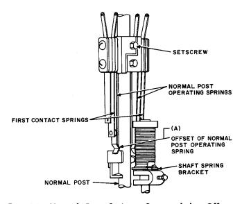
Fig. 14—Normal Post Springs Operated by Offset Shaft Spring Bracket
