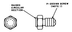
Fig. 6—Normal Post Spring Assembly Mounting Screw
