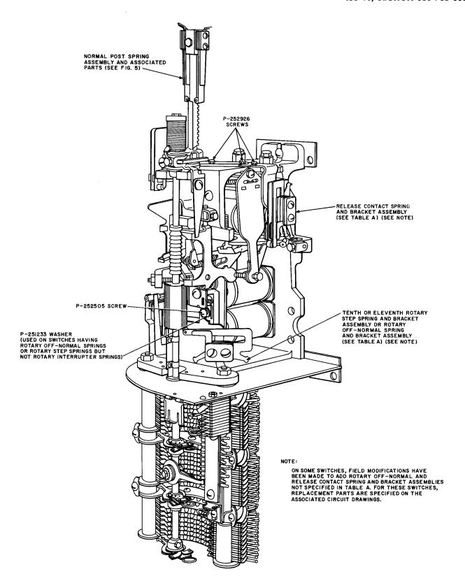
Fig. 2—Contact Spring Assemblies, Test Jack Assemblies, and Associated Parts of 197-Type Switch as Viewed From the Right Side
