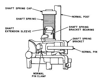
Fig. 16—Helical-Type Shaft Spring Assembly
