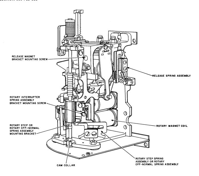
Fig. 10—Parts of 197-Type Switch as Viewed From the Right Side
