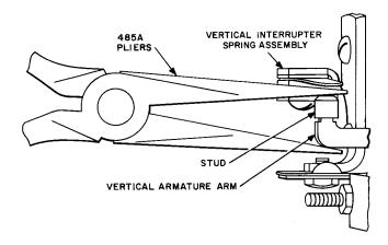
Fig. 8—Method of Replacing Stud on Vertical Armature
