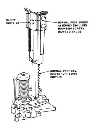
Fig. 5—Normal Post Spring Assembly and Associated Parts
