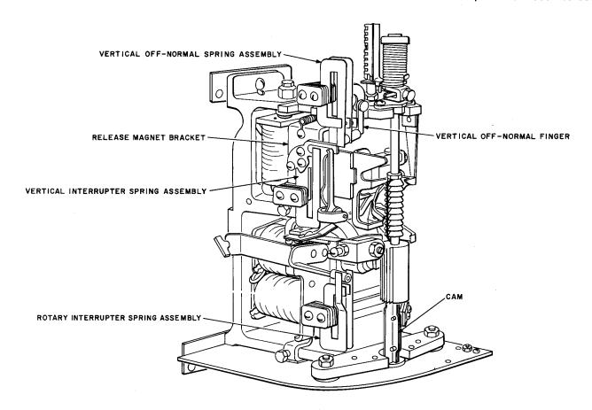
Fig. 9—Parts of 197-Type Switch as Viewed From the Left Side
