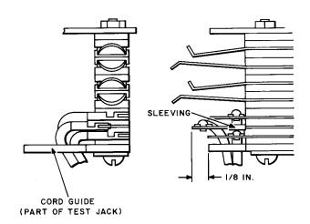
Fig. 17—Method of Dressing and Connecting Wiper Cords
