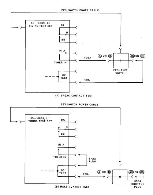
Fig. 16—Test Arrangement for 223-Type Switch Timing Tests
