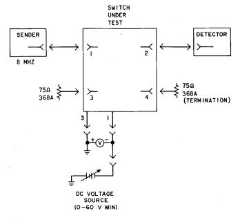
Fig. 19-Insertion and Isolation Loss/Test Circuit
