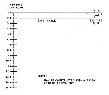
Fig. 7—Power Cable to Connect 35-Type Test Set to J68333 Test Bench
