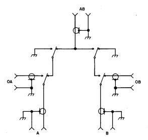
Fig. 5—223A Coaxial Switch Schematic Shown in Normal (Released Condition)
