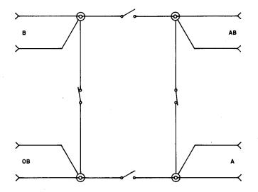
Fig. 6—223E Coaxial Switch Schematic Shown in Normal (Released Condition)
