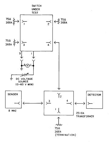
Fig. 20—Return Loss Test Circuit
