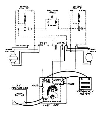
Fig. 9 – Test Connections for Relay "B" With Transformer
