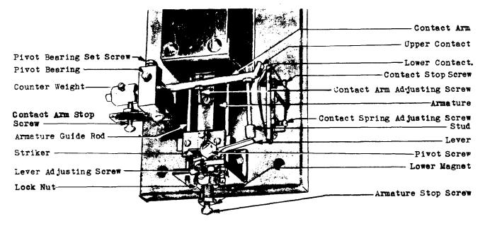
Fig. 3 – Voltage Relay Details
