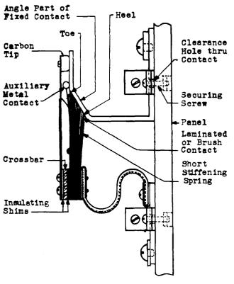
Note: The separation between leaves of the brush is shown exaggerated and is not usually obtainable in practice.
