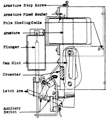
Fig. 12 – Operating, Tripping and Latch Mechanism
