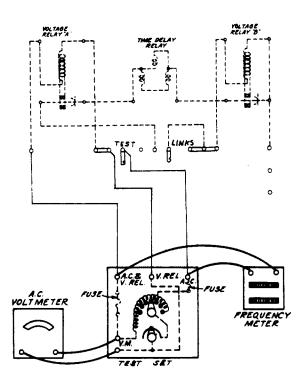
"ig. 6 - Test Connections for Relay "A" Without Transformer
