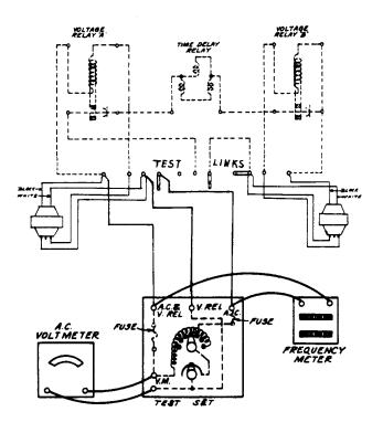
Fig. 8 – Test Connections for Relay "A" With Transformer
