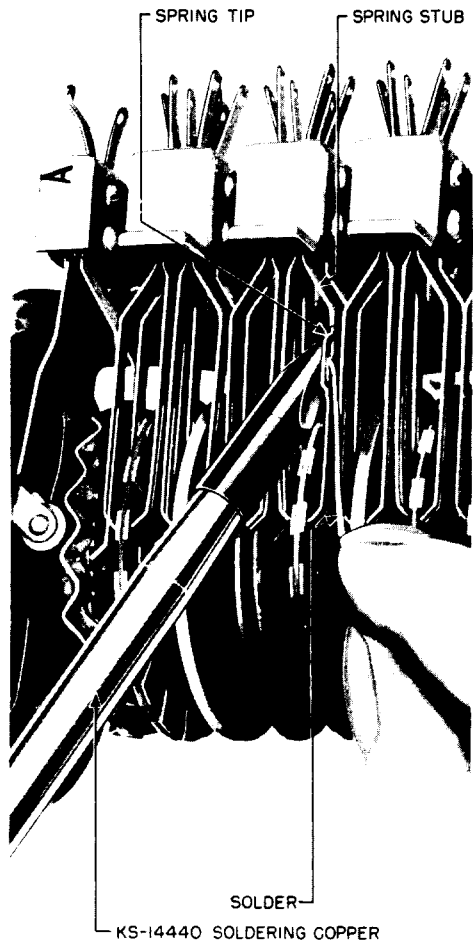
Fig. 3 - Method of Soldering Spring Tips
