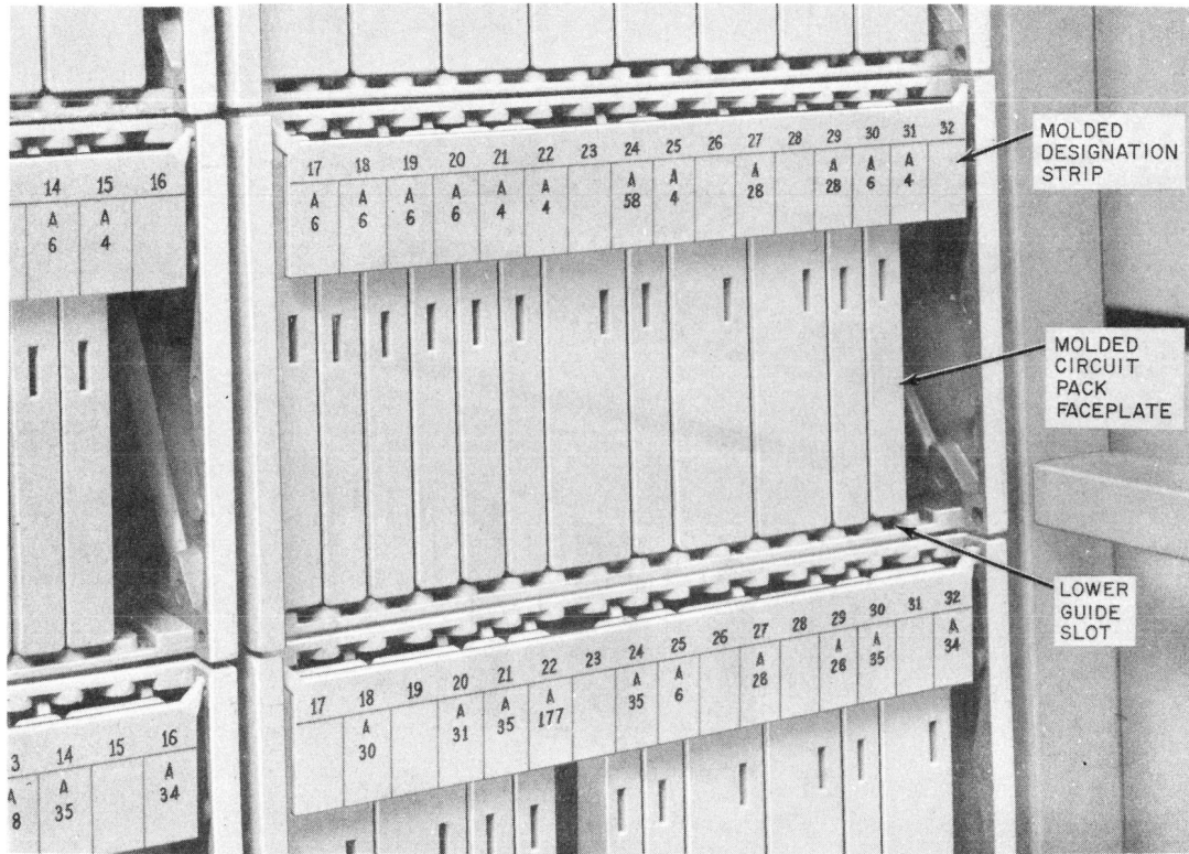
Fig. 4—Molded Circuit Faceplate and Front of Apparatus Mounting With Hinged Description Strip in Normal Position
