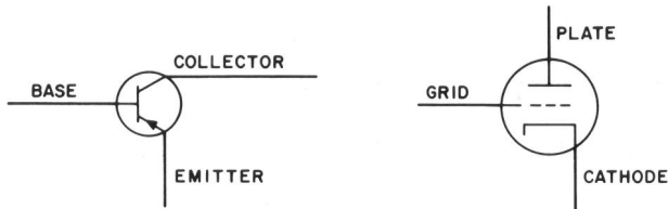
Fig. 1—Comparison of Transistor and Vacuum Tube
