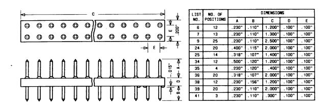
♦Fig. 24—KS-21307, L6, L7, L9, L24, L25, L34, L35, L36, L38, L39, or L41, Connector€
