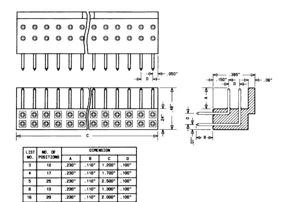
♦Fig. 23—KS-21307, L3, L4, L5, L8, or L16, Connector♥
