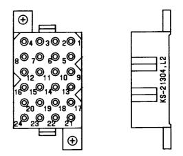
♦Fig. 9—KS-21304, L2, Connector Pin Contact♥
