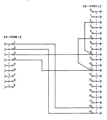
The P4AP cord includes one KS-19088, L5, connector and one KS-14460, L2, plug. The cord initially was intended for use for inservice maintenance of 240-type amplifiers in the type N Carrier Telephone Systems.
