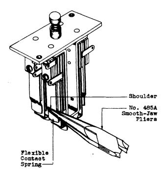
Fig. 8 – Method of Adjusting Tip of Flexible Contact Spring
