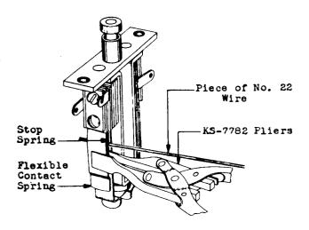
Fig. 9 - Method of Adjusting Flexible
