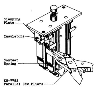
Fig. 7 – Method of Adjusting for Contact Separation
