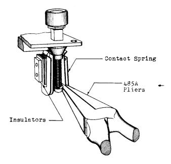
Fig. 5 - Method of Adjusting Contact Springs
