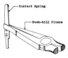
Fig. 4 - Method of Adjusting for Contact Pressure
