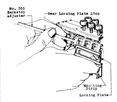
Fig. 14 — Method of Adjusting Rear Locking Plate
