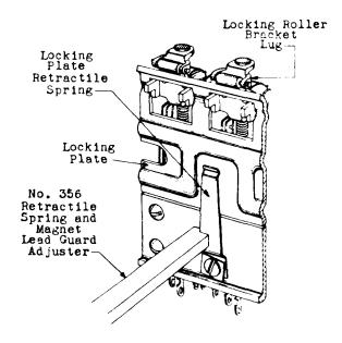
Fig. 12 — Method of Adjusting Locking Plate
