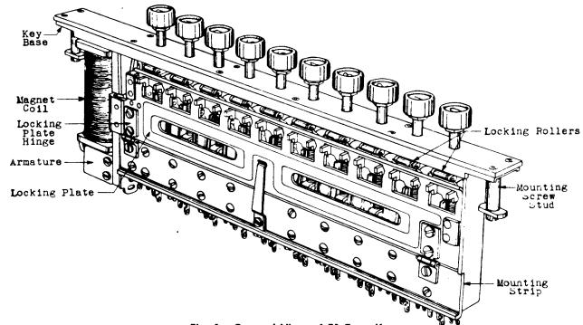
Fig. 1 - General View of E1 Type Key
