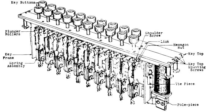
Fig. 2 - General View of E2 Type Key
