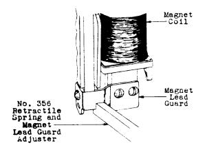
Fig. 15 – Adjustment of Gap Between Armature and Magnet Pole-Piece
