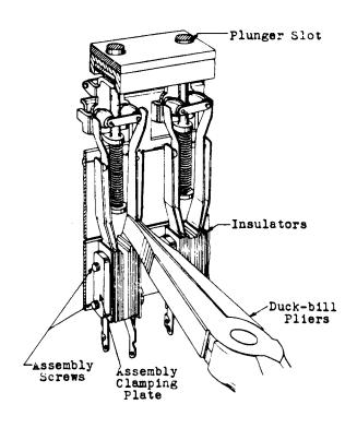
Fig. 16 - Method of Adjusting for Contact Pressure
