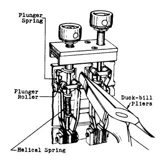
Fig. 17 - Method of Adjusting for Spring Clearance
