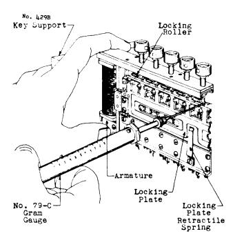
Fig. 11 — Measurement of Locking Plate
