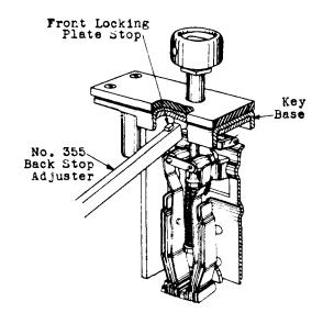
Fig. 13 — Method of Adjusting Front Locking
