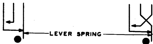
Fig. 2 - Special Make-before-Break Contact Springs
