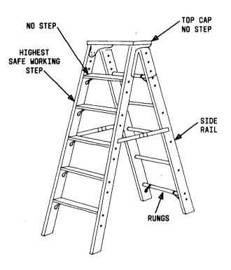
Fig. 3 — Stepladder (4 feet or larger) Maximum Working Height
