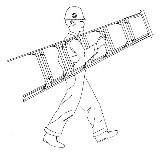
Fig. 4 — Carrying a Stepladder Under 8 Feet in Length
