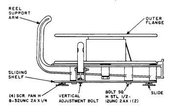
Fig. 5—Wire Reel Assembly
