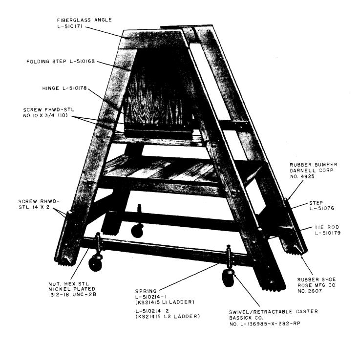
Fig. 1—KS-21415 L1 Rolling Platform Ladder (Folding Step Stored Position)
