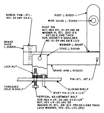
Fig. 6—Automatic Brake Assembly
