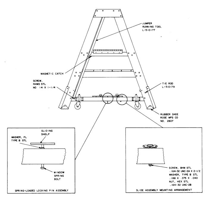
Fig. 7—KS-21415 L2 Rolling Platform Ladder (Magnetic Catch, Sliding Shelf Locking and Mounting Arrangements)
