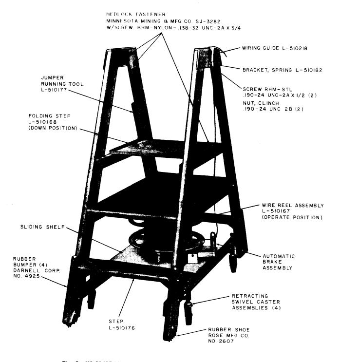
Fig. 2—KS-21415 L2 Rolling Platform Ladder (Wire Reel Operate Position)
