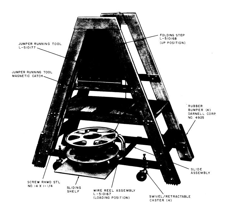
Fig. 3—KS-21415 L2 Rolling Platform Ladder (Wire Reel Loading Position)
