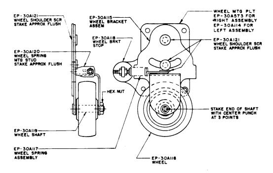
Fig. 6—Platform and Portable-Type Rolling Ladder Wheel Assemblies
