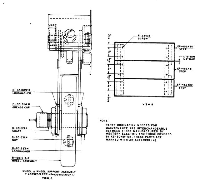
Fig. 3—Views of Portable-Type Rolling Ladder
