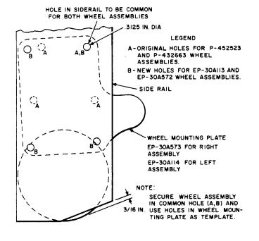
Fig. 7—Modification of Side Rails of Portable-Type Rolling Ladder for Wheel Assembly Replacement
