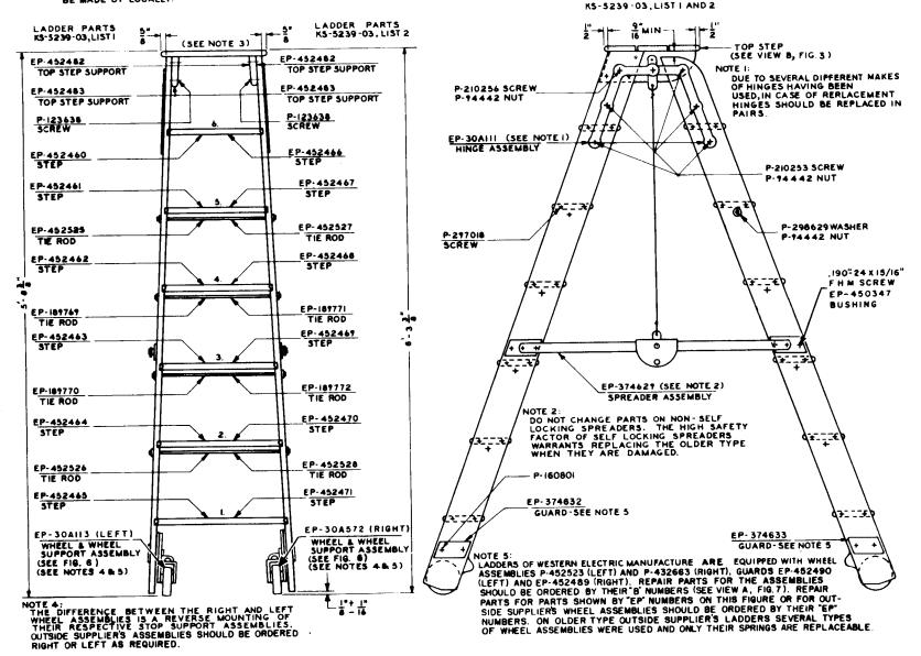
Fig. 2—Portable-Type Rolling Ladder
