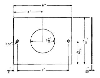
Fig. 7 - P-416920 Spacer (Green Blotting Paper) (Inches)
