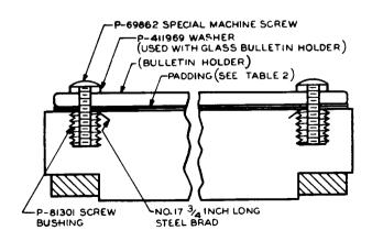
Fig. 1 - Bulletin Holder Mounted on Shelf
